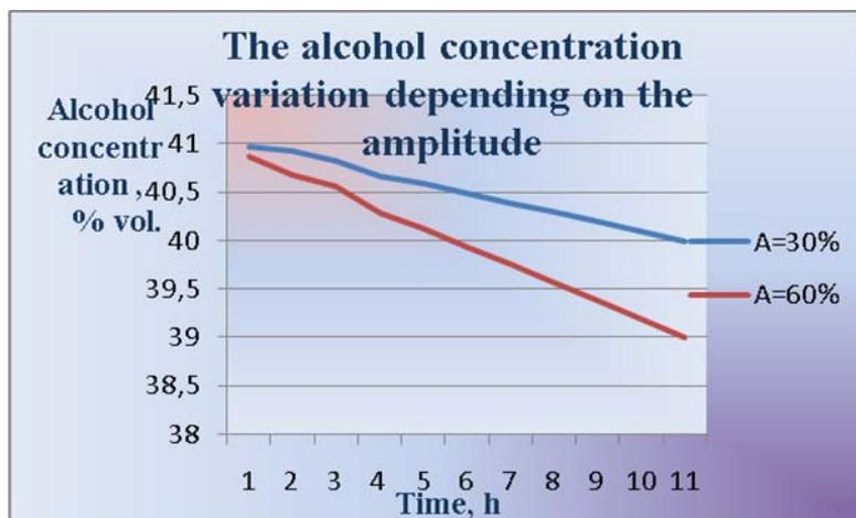
Fig. 5. Alcohol variation according to amplitude.
