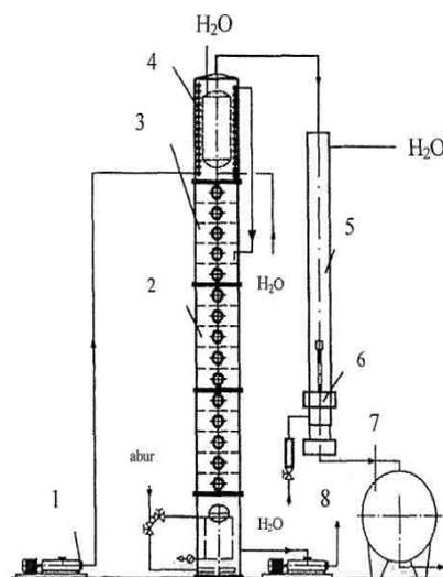
Fig. 1. *Distillation and rectification equipment (continuous installation).*
