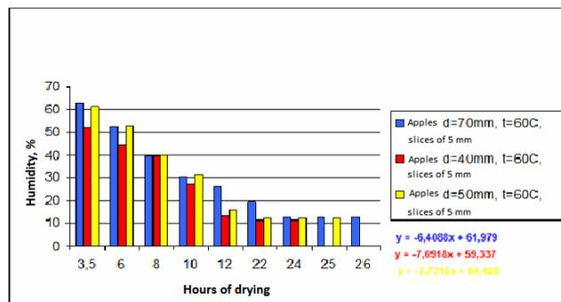
Fig. 14. The influence of the initial dimension of the sample on drying duration in the case of apples slices of 5mm thickness, dried at a temperature of 60°C
