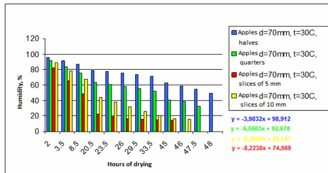
Fig. 13. The influence of the system of slicing on the drying time in the case of apples with a diameter of 70mm dried at a temperature of 30°C
