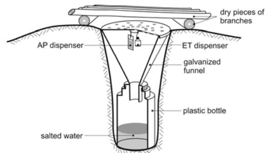
Fig. 3. The design of the traps used in the experiment
