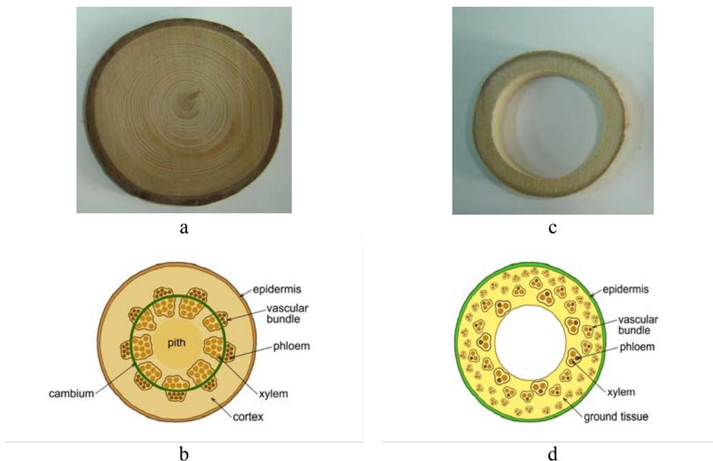
Fig. 4. *General macroscopic and microscopic appearance of wood and Bamboo*
