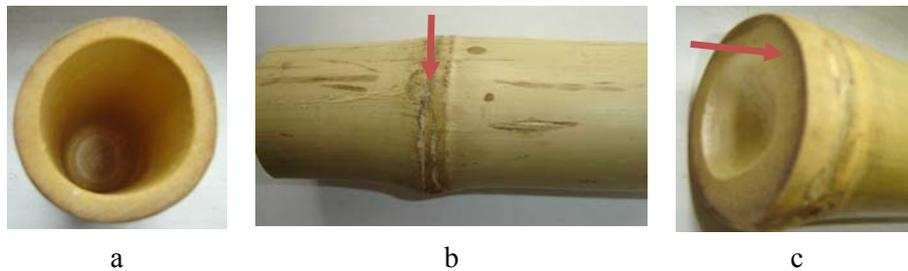
Fig. 3. *Hollow stem (a) and the solid node area (b,c)*
