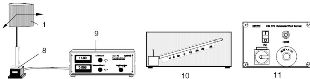
Fig. 5. The measurement system with manometer tube and control panel [6]
