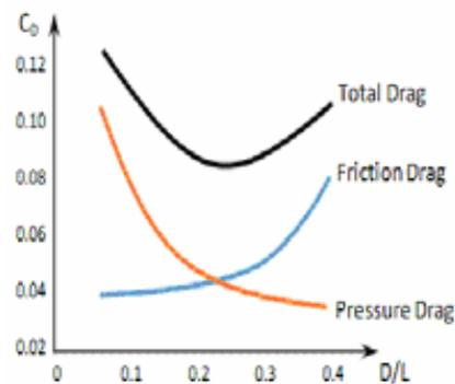
Fig. 1. Trade-off relationship between pressure drag and friction drag [1]
