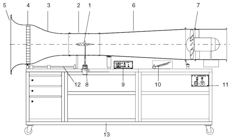
Fig. 4. The structure of aerodynamic wind tunnel [6]
