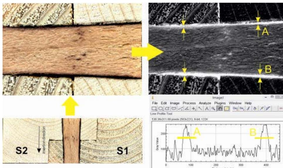
Fig. 7. The contact area between wood dowels and spruce - maple wood material
