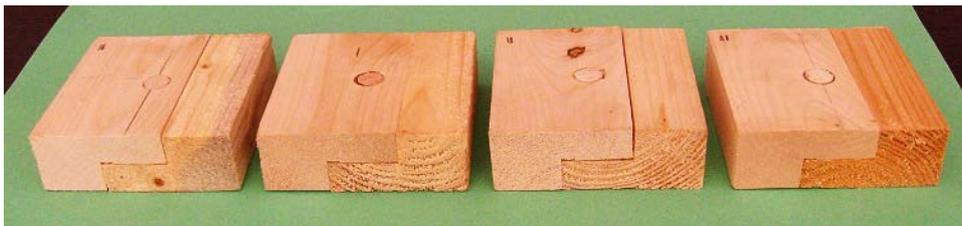
Fig. 3. The structures obtained by insertion of dowels first in maple and then in spruce
