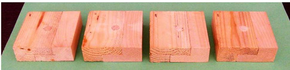
Fig. 4. The structures obtained by insertion of dowels first in spruce and then in maple
