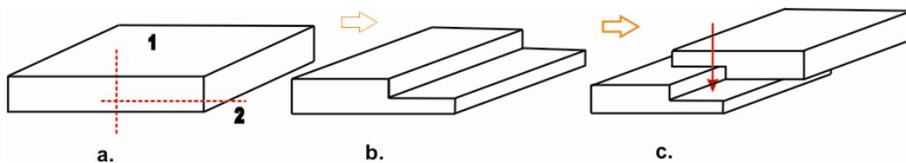
Fig. 1. The main procedure for obtaining the samples: a. cutting; b. profiling; c. joining
