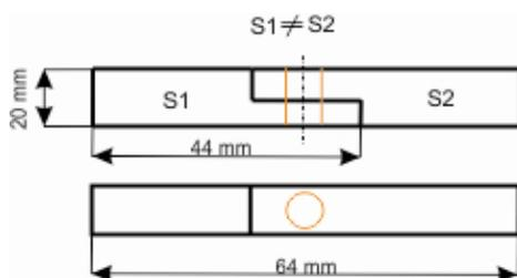
Fig. 2 Dimensions and type of structures proposed for joints without adhesive
