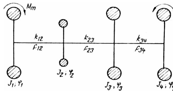
Fig. 1. The dynamic model of the transmission mechanism between tractor and baler
