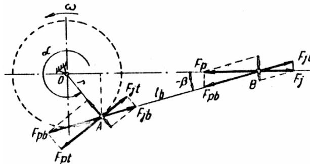
Fig. 2. Representing the kinematics of the crank mechanism
