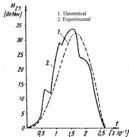
Fig. 3. Comparison between the torsion torques values to PTO shaft determined by calculation and experimental methods
