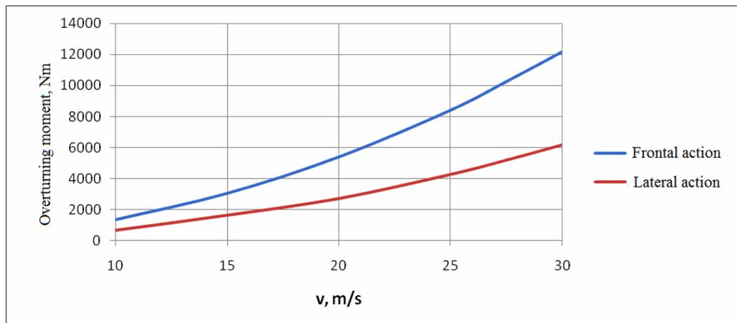
Fig. 14. Variation of the overturning moment of the greenhouse
