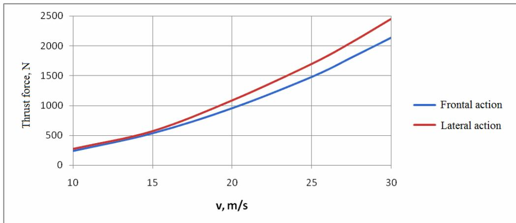
Fig. 12. *Variation of the thrust force of the greenhouse*
