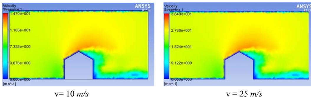
Fig. 10. Visualizing the air flowing in the vertical middle section of the area in the case of lateral wind action
