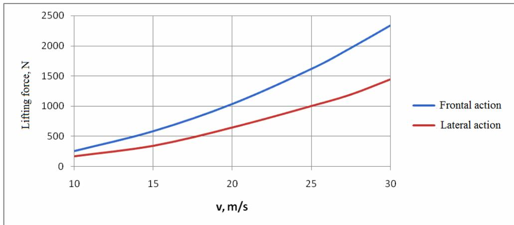
Fig. 13. Variation of the lifting force of the greenhouse
