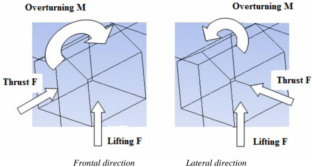
Fig. 11. *The scheme of the thrust and lifting forces and respectively of the overturning moment acting on the greenhouse depending on the speed and direction of wind action*
