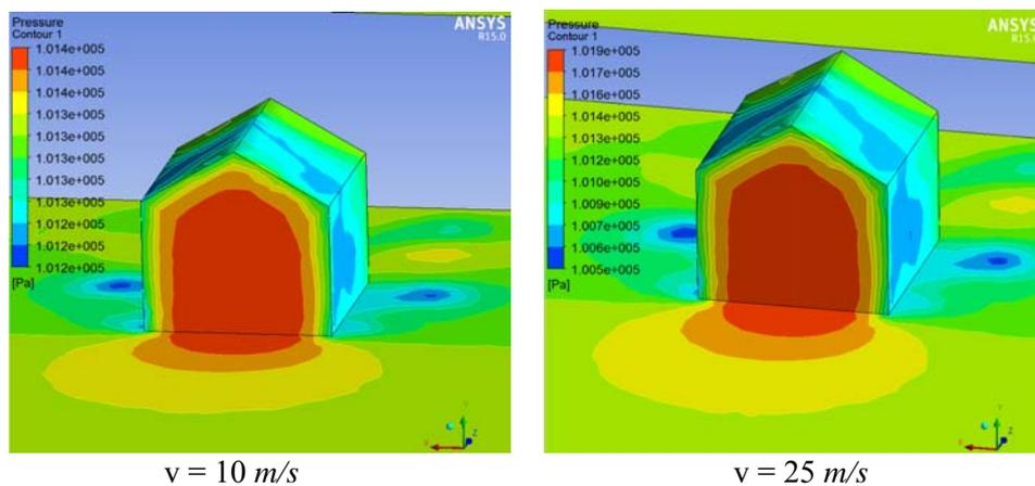
Fig. 5. *The maximum pressure of the wind on the frontal surface*
