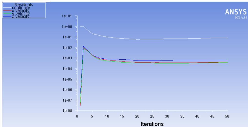
Fig. 3. *The stabilisation of the residual error considering the frontal wind action*
