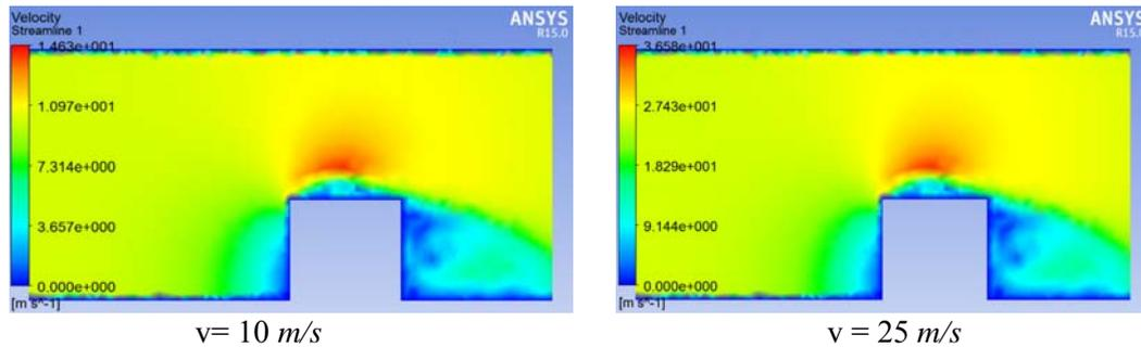
Fig. 9. Visualizing the air flowing in the vertical middle section of the area in the case of frontal wind action
