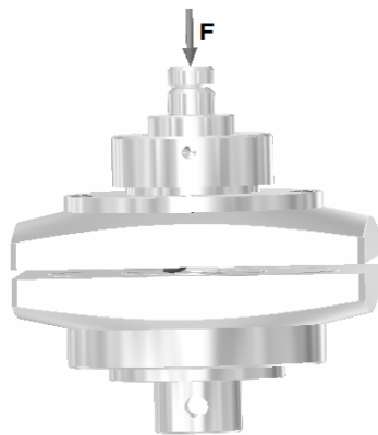
Fig.1. Uniaxial compression of wheat grain between two parallel plates [5],[8]
