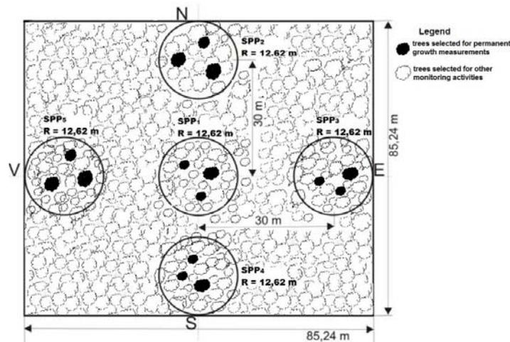
Fig. 2. *Intensive monitoring Level II plot design and the location of the 15 trees selected for permanent growth measurements*
