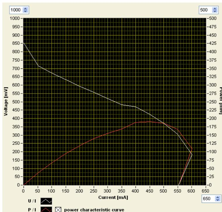
Fig. 5. *The characteristic curves of the fuel cell at the end of tests*
