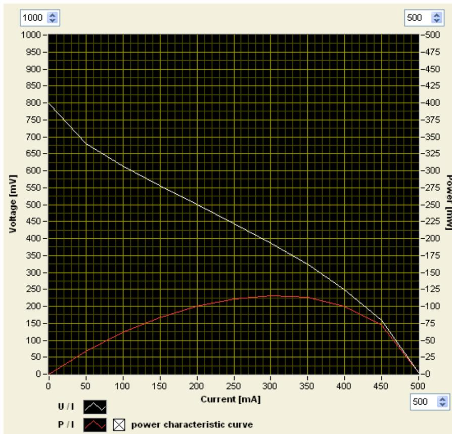
Fig. 2. *The characteristic curves of one PV panel*
