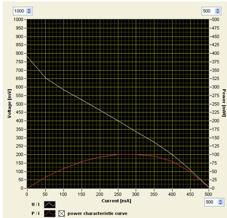
Fig. 4. *The characteristic curves of the fuel cell at the beginning of tests*
