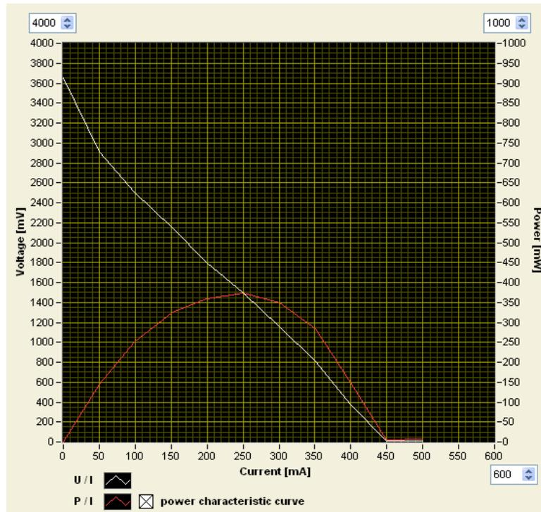
Fig. 3. *The characteristic curves of the wind turbine*
