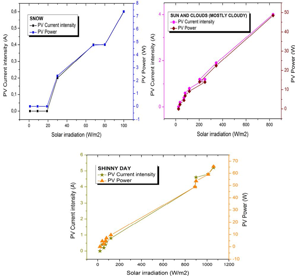
Fig. 2. The influence of the solar irradiation on the PV parameters in different weather conditions
