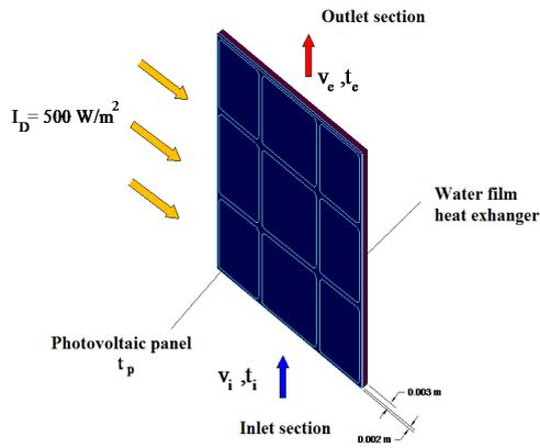
Fig. 1. The model of PV panel and heat exchanger studied in ANSYS-Fluent
