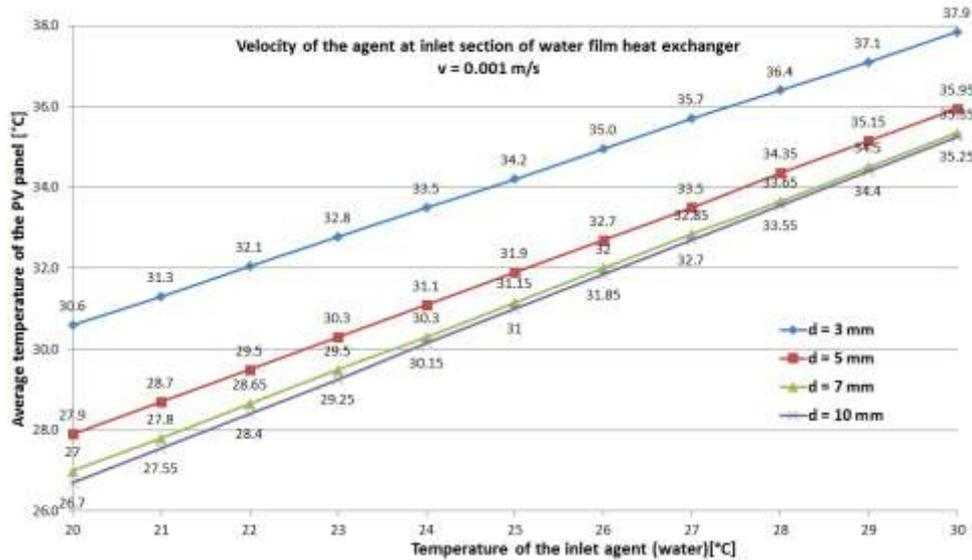
Fig. 2. Variation of average temperature of the PV panel depending on the width of water film and inlet temperature of heat transfer agent
