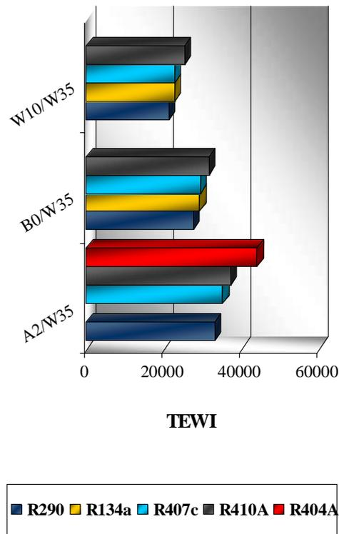
Fig. 7. The values of index TEWI for various refrigerants and different types of heat pumps
