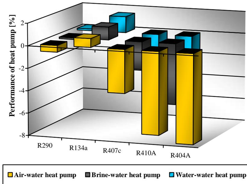
Fig. 6. The performance of different heat pumps as compared with those using R-22
