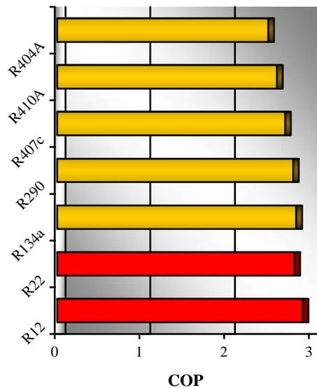
Fig. 3. COP values for different refrigerants for an air-water heat pump (A2/W35)
