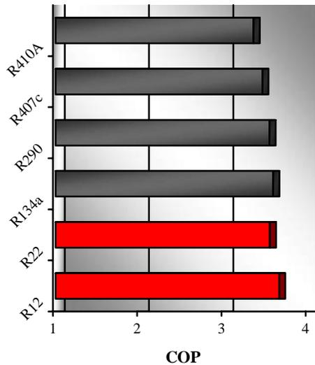
Fig. 5. COP values for different refrigerants for a brine-water heat pump (B0/W35)
