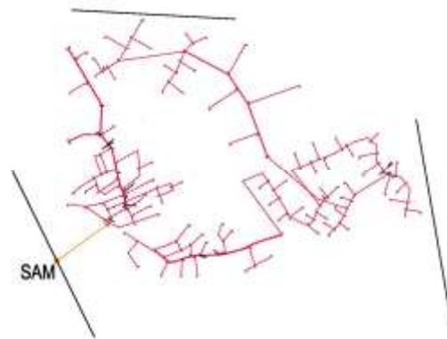
Fig. 2. *Constructive variant 2 of natural gas distribution network*
