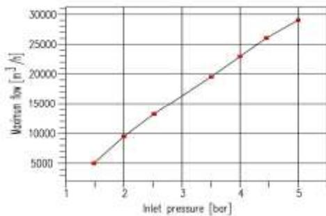
Fig. 7. *The maximum flow variation depending on the inlet pressure*
