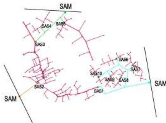
Fig. 1. *Constructive variant 1 of natural gas distribution network*
