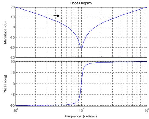
Fig. 9. Bode diagram of the behavior of a high frequency capacitor
