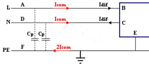
Fig. 12. Equipment affected by emissions on the low voltage grid
