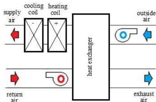
Fig. 1. Schematic diagram of an air handling unit
