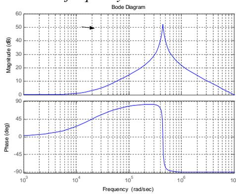
Fig. 11. Bode diagram of the behavior of a high frequency inductor
