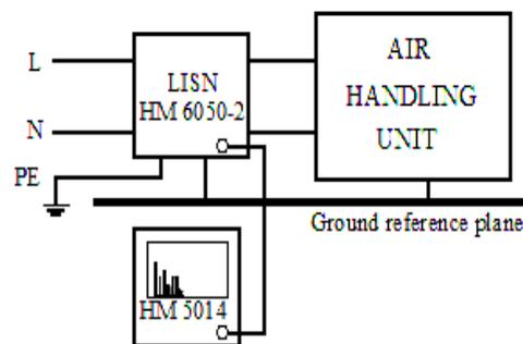
Fig. 2. The schematic test setup for conducted interference
