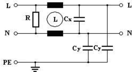
Fig. 5. Typical topology of mains filter
