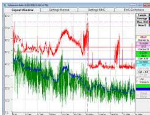
Fig. 3. *Conducted interferences of the AHU in linear scale*
