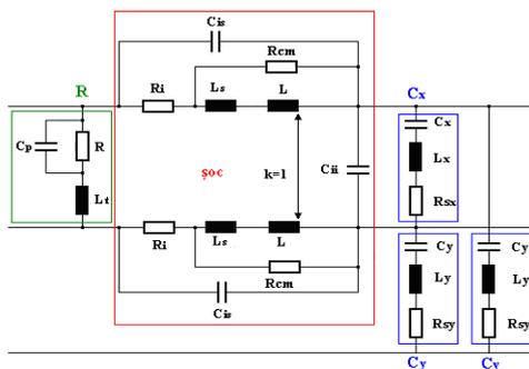
Fig. 14. Equivalent schematics of an EMI filtering cell
