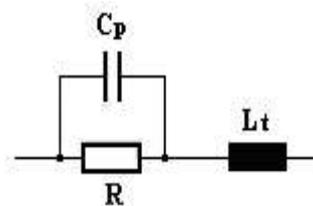
Fig. 6. Equivalent schematics of a high frequency resistor
