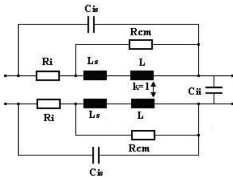
Fig. 13. Common mode choke
