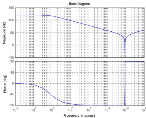
Fig. 7. Bode diagram of the behavior of a high frequency resistor
