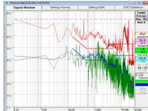
Fig. 4. *Conducted interferences of the AHU in logarithmic scale*
