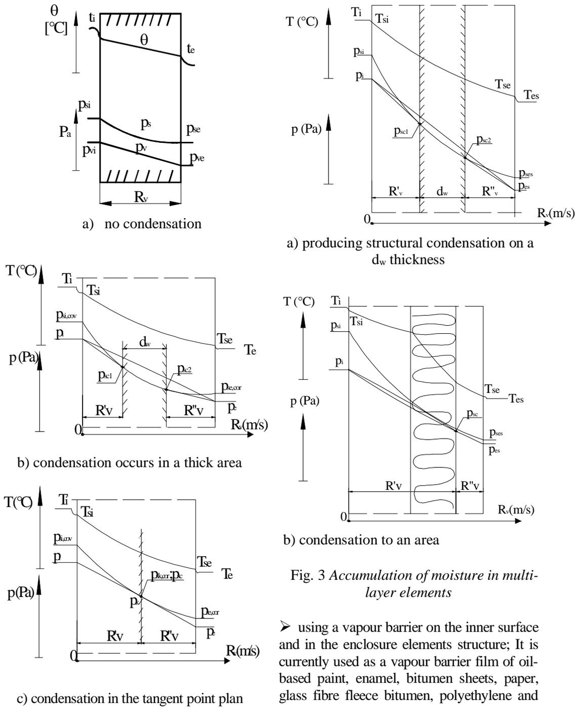
Fig. 2. *Graphical analysis of the condensation risk to monolayer elements*
