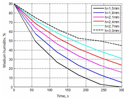
Fig. 2. Evolution versus time and the average residual moisture of chips for various thickness "h" of the potato slices (frying oil temperature,  $u = 180^\circ\text{C}$ )
