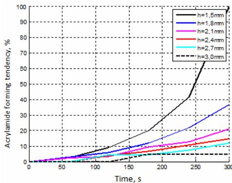
Fig. 3. Evolution versus time and trend of Acrylamide formation (TA) in the chips for various thickness "h" of the potato slices (oil temperature  $T_u = 180^\circ\text{C}$ )
