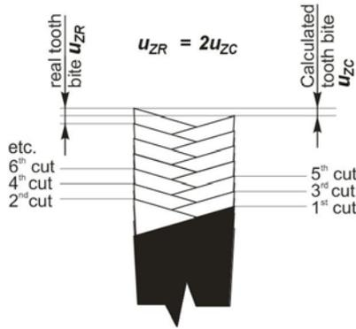
Fig. 5. The cutting succession as a result of the cutting teeth geometry.
