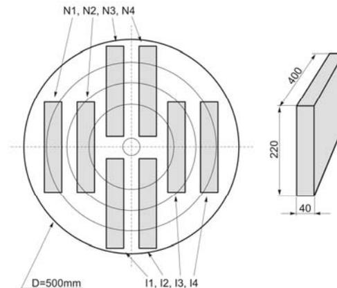
Fig. 1. Cutting scheme for obtaining the wood specimens.
