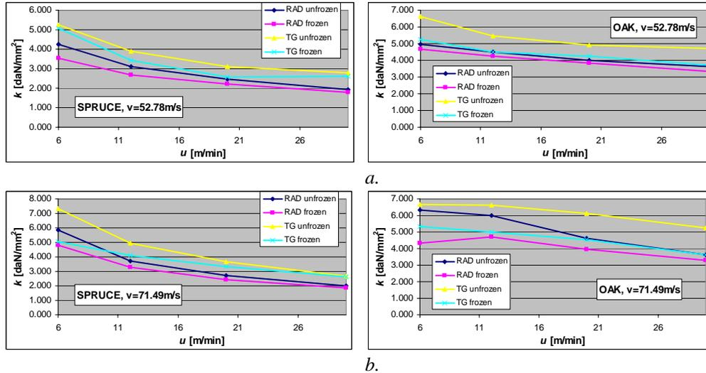
Fig. 7. Comparative values of the specific resistance to cutting ( $k$ ) during the sawing of frozen and unfrozen spruce and oak wood.
