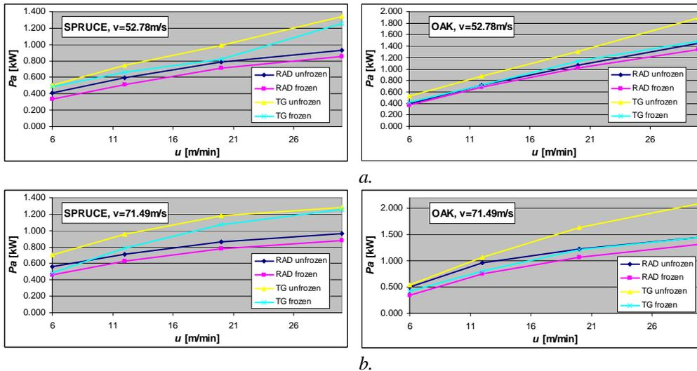
Fig. 6. Comparative values of the consumed power ( $P_a$ ) during the sawing of frozen and unfrozen spruce and oak wood.
