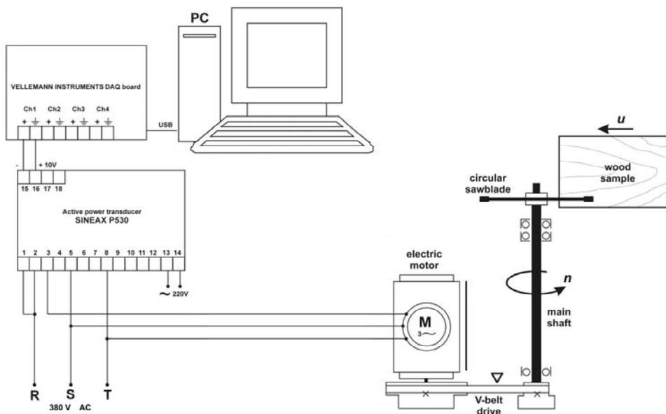
Fig. 3. Working set-up.
