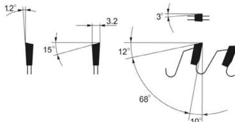
Fig. 4. The parameters of the circular blade teeth.
