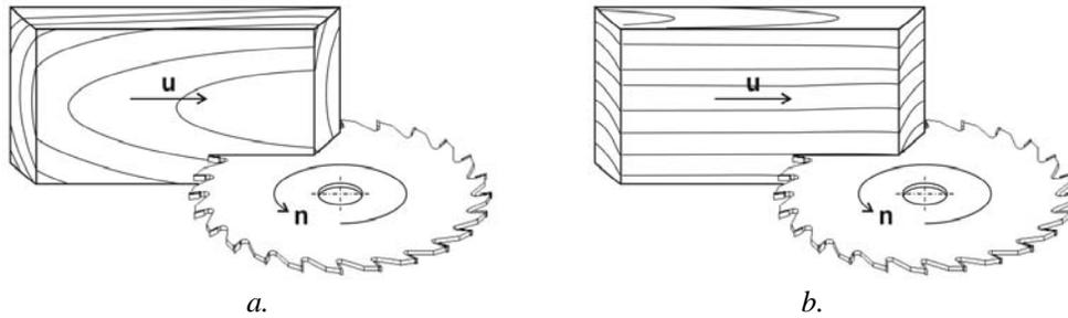
Fig. 2. Working schemes: *a*-radial cutting plane; *b*-tangential cutting plane.
