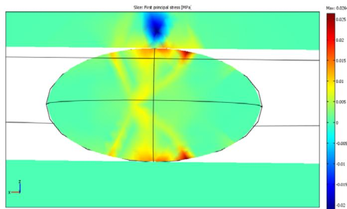
Fig. 4. *Values obtained during the first compressions to crushing of the wheat grain*
