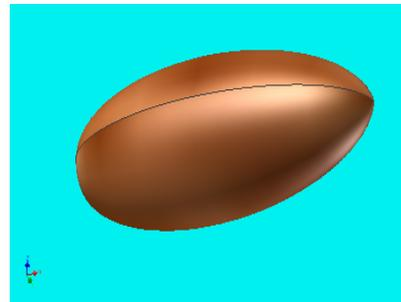
Fig. 2. Geometry of the wheat grain
