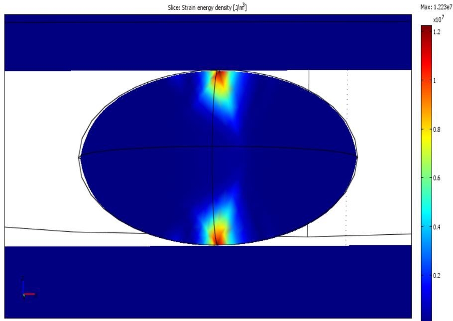
Fig. 7. The energy values obtained as a consequence of the grinding process by wheat grain crushing  $[J/m^3]$
