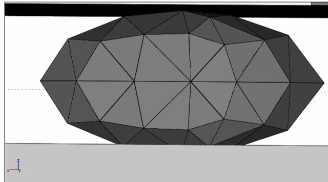
Fig. 3. *Digitations of a wheat grain in finite element*
