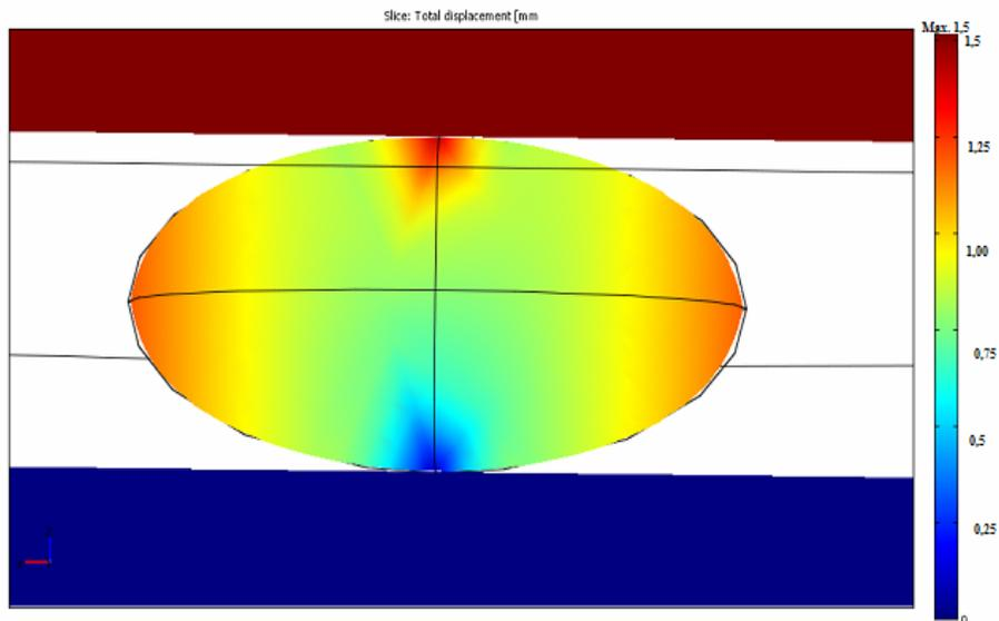
Fig. 6. Grain deformations on crushing direction [mm]
