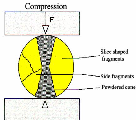
Fig. 1. Model of a ferric grain stressed to compression [6]
