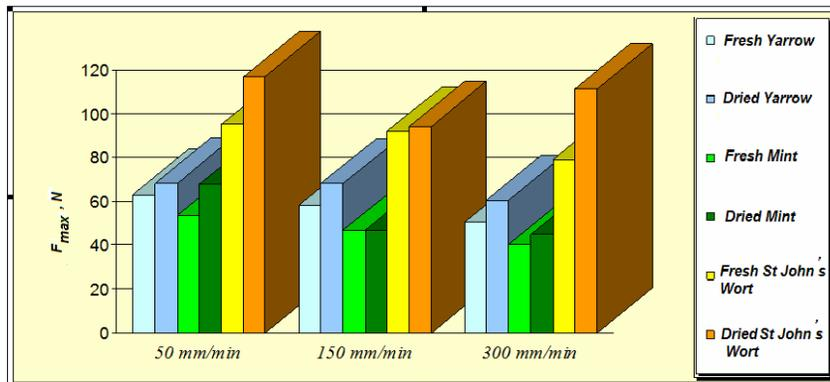
Fig. 7. Variation of the cutting resistance force values obtained when cutting the three species of herbs with a straight edge knife and sharpening angle of 45°
