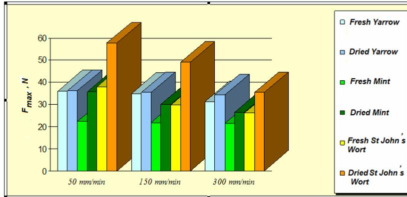
Fig. 5. Variation of the cutting resistance force values obtained when cutting the three species of herbs with a straight edge knife and sharpening angle of 15°
