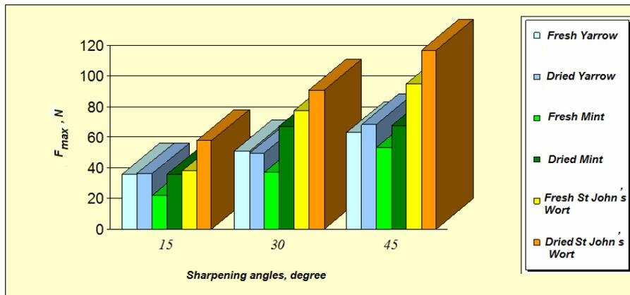
Fig. 8. Variation of the cutting resistance force values obtained when cutting the three species of herbs with a straight edge knife and sharpening angles of 15, 30 and 45°, at a speed of 50 mm/min
