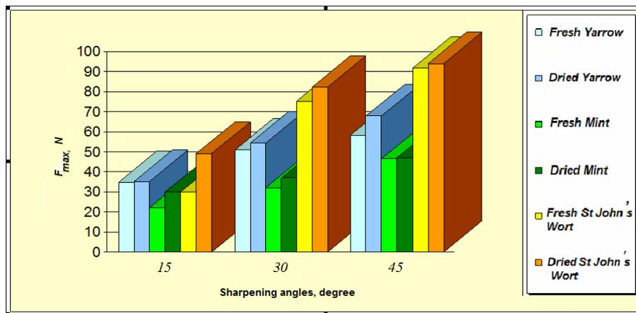
Fig. 9. Variation of the cutting resistance force values obtained when cutting the three species of herbs with a straight edge knife and sharpening angles of 15, 30 and 45°, at a speed of 150 mm/min
