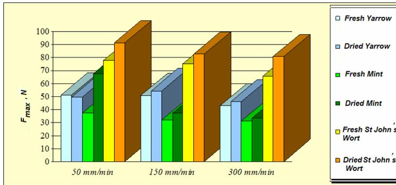
Fig. 6. Variation of the cutting resistance force values obtained when cutting the three species of herbs with a straight edge knife and sharpening angle of 30°
