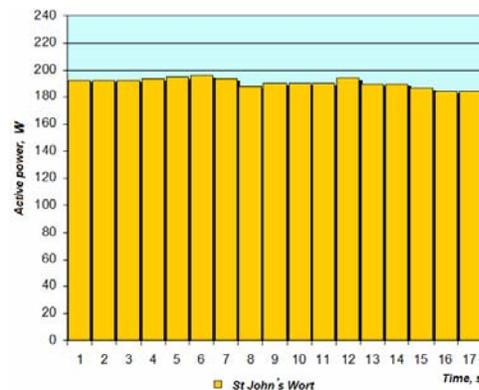
Fig. 11. Variation of active power in the process of cutting fresh *St. John's wort*
