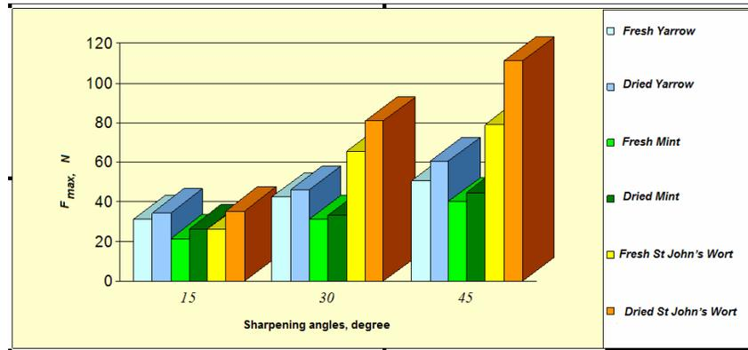
Fig. 10. Variation of the cutting resistance force values obtained when cutting the three species of herbs with a straight edge knife and sharpening angles of 15, 30 and 45°, at a speed of 300 mm/min
