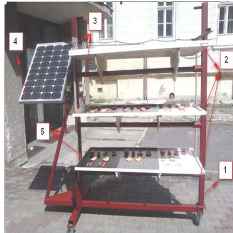
Fig. 3. *Stand for research of carrots drying with solar energy*
