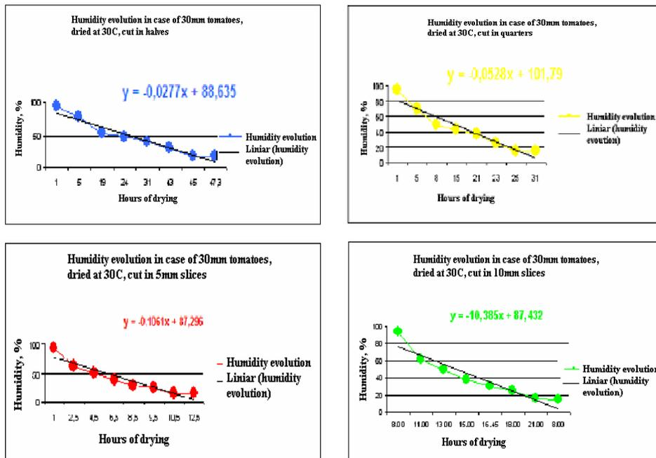
Fig. 7. *Drying curves and regression equations for each slicing system*
