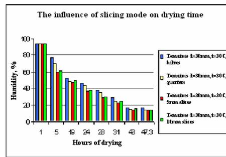
Fig. 6. *The influence of the slicing mode on drying time in the case of tomatoes with a 30 mm diameter*
