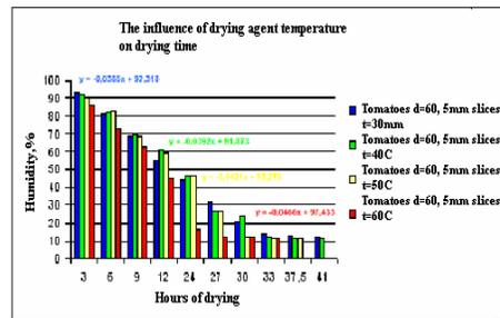
Fig. 9. *The influence of the drying agent temperature on drying time in the case of tomatoes with a 60 mm diameter*
