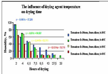
Fig. 8. *The influence of the drying agent temperature on drying time in the case of tomatoes with a 30 mm diameter*
