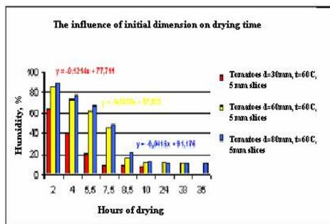
Fig. 11. The influence of the initial dimension of samples on drying time for tomatoes with a 30, 60 and 80 mm diameter, dried in slices with a 5 mm thickness
