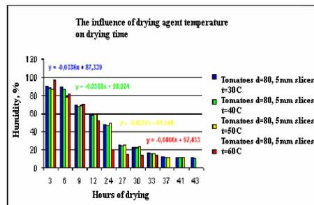
Fig. 10. *The influence of the drying agent temperature on drying time in case of tomatoes with an 80 mm diameter*
