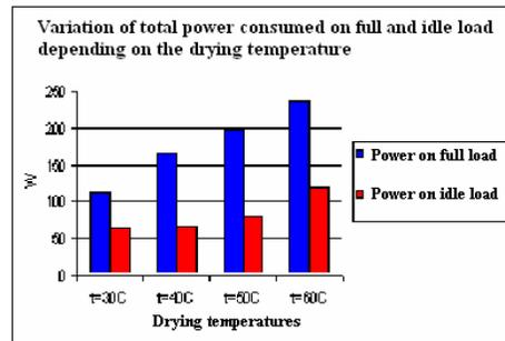
Fig. 5. Variation of total consumed power and idle depending on drying temperature
