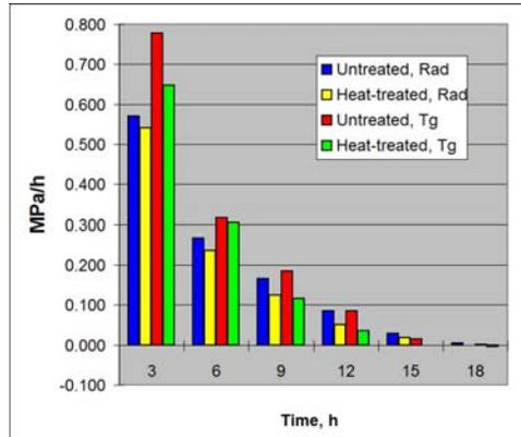
Fig. 4. Speed evolution of swelling pressure at untreated and heat-treated ash wood moisturized by water immersion (averages calculated on 3h intervals, first 18h).
