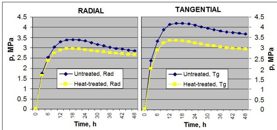
Fig. 3. *Evolution of swelling pressure at untreated and heat-treated ash wood moisturized by water immersion (averages).*
