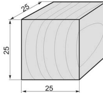
Fig. 1. *Scheme of the wood samples used for the experiments*
