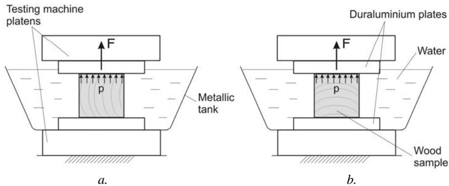
Fig. 2. Scheme of the experimental device for measuring the swelling forces:
