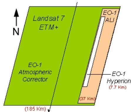
Fig. 2. *The size of satellite images taken with the ALI sensor*
