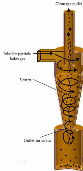
Fig. 1. Schematic diagram of a reverse flow cyclone separator
