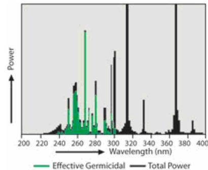
Fig. 7. MP/HP mercury lamp relative spectral power distribution curve [10]
