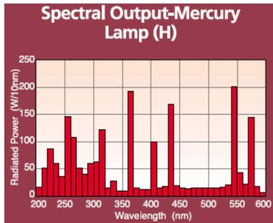
Fig. 5. Typical spectral output from a Mercury Lamp [12]
