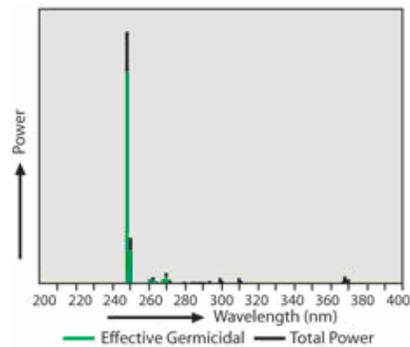
Fig. 6. LP mercury lamp relative spectral power distribution curve [10]
