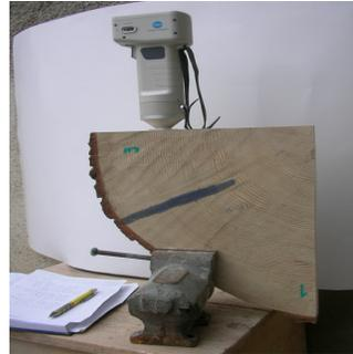
Fig. 1. *The colour measurement on radial side of wood using CR-400 colorimeter*
