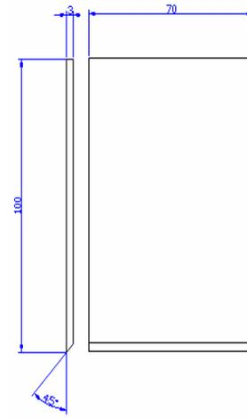
Fig. 4. *Graphic representation of the cutting knife with the sharpening angle of 45°*
