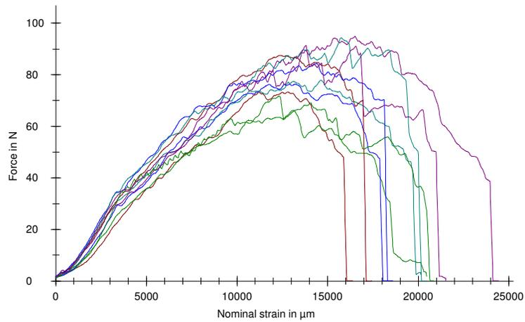
Fig. 7. Variation of cutting resistance for the knife with sharpening angle of 30°
