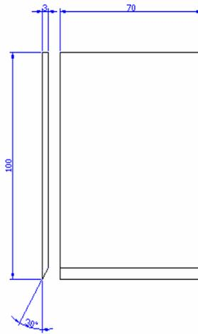
Fig. 3. *Graphic representation of the cutting knife with the sharpening angle of 30°*
