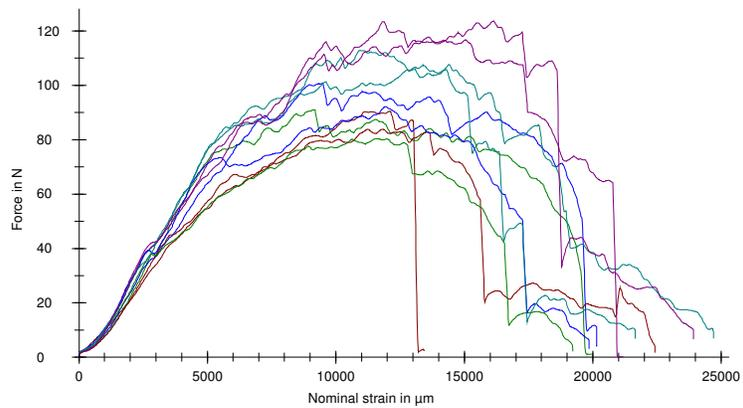
Fig. 8. Variation of cutting resistance for the knife with sharpening angle of 45°
