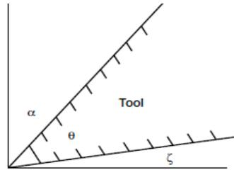
Fig. 1. Sharp tool represented by a wedge of included angle  $\theta$ . The rake angle of the tool is  $\alpha$ ; the clearance (relief) angle is  $\zeta$
