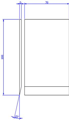
Fig. 2. *Graphic representation of the cutting knife with the sharpening angle of 15°*
