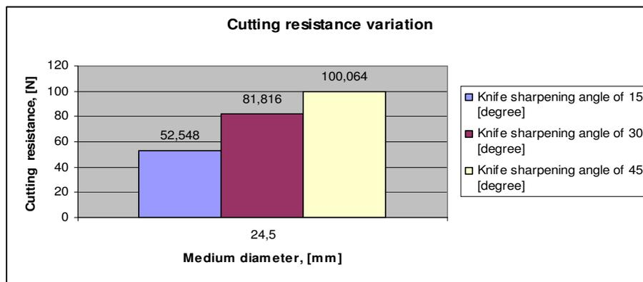
Fig. 9. Variations of cutting resistance force at different values of the knife sharpening angle
