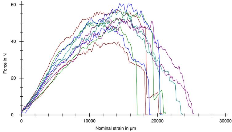
Fig. 6. Variation of cutting resistance for the knife with sharpening angle of 15°
