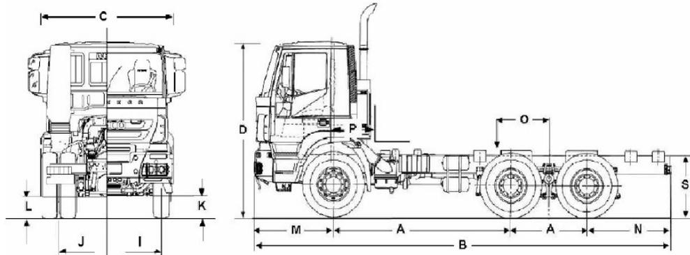
Fig. 1. Technical schema for a truck-train having a simple axle in the front part and a double axle in the rear part
