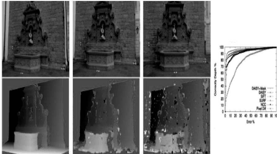
Fig. 1. Comparing different descriptors with ground truth (first laser scan, second DAISY, third NCC) [6]
