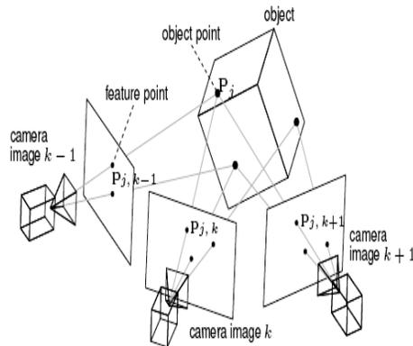
Fig. 2. The projection of a 3D object point  $P_j$  in the camera image [8]
