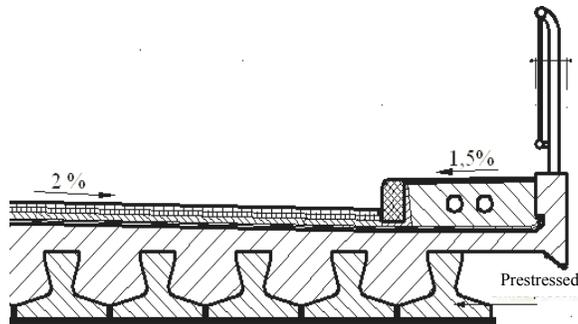
Fig. 3. Prestressed concrete T-beams decks
