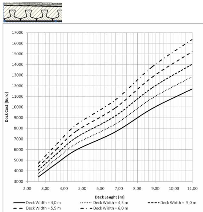
Fig. 4. The cost of T-beams decks, in function of width and length
