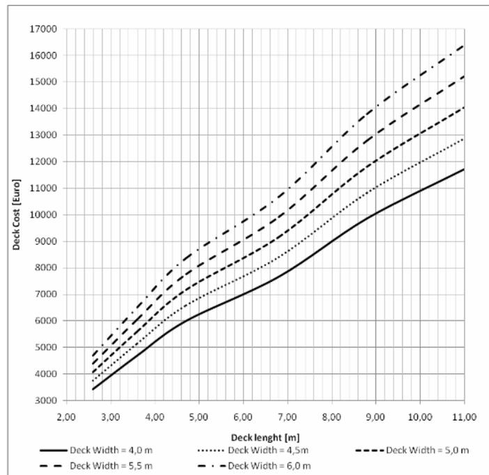
Fig. 2.  $\Pi$ -Beam deck costs, in function of width and length
