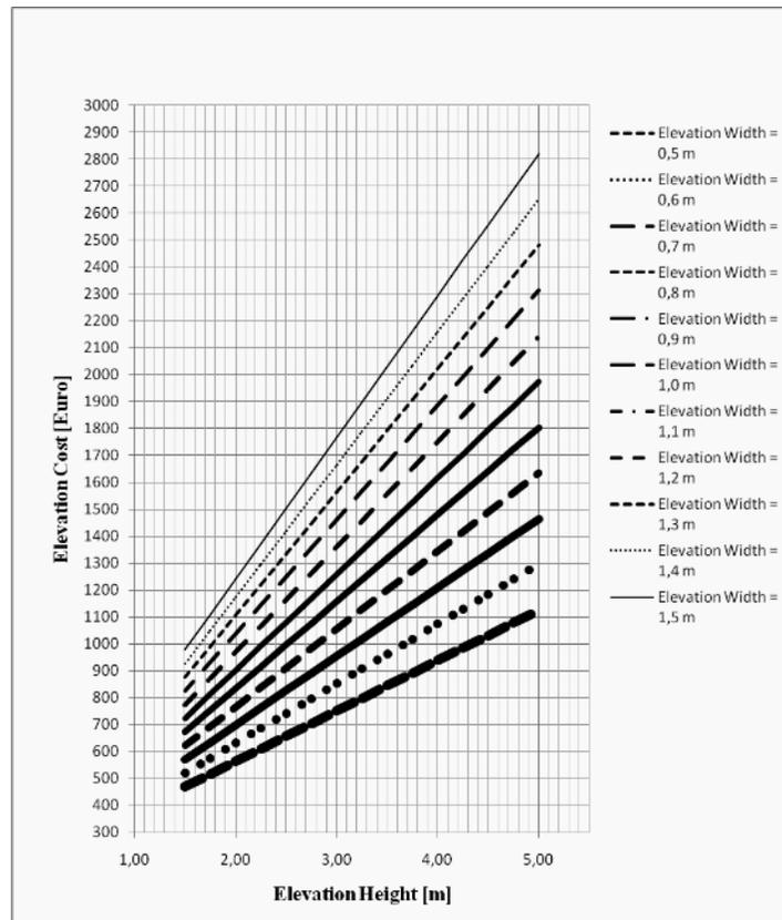
Fig. 7. Elevations costs in function of dimensional elements
