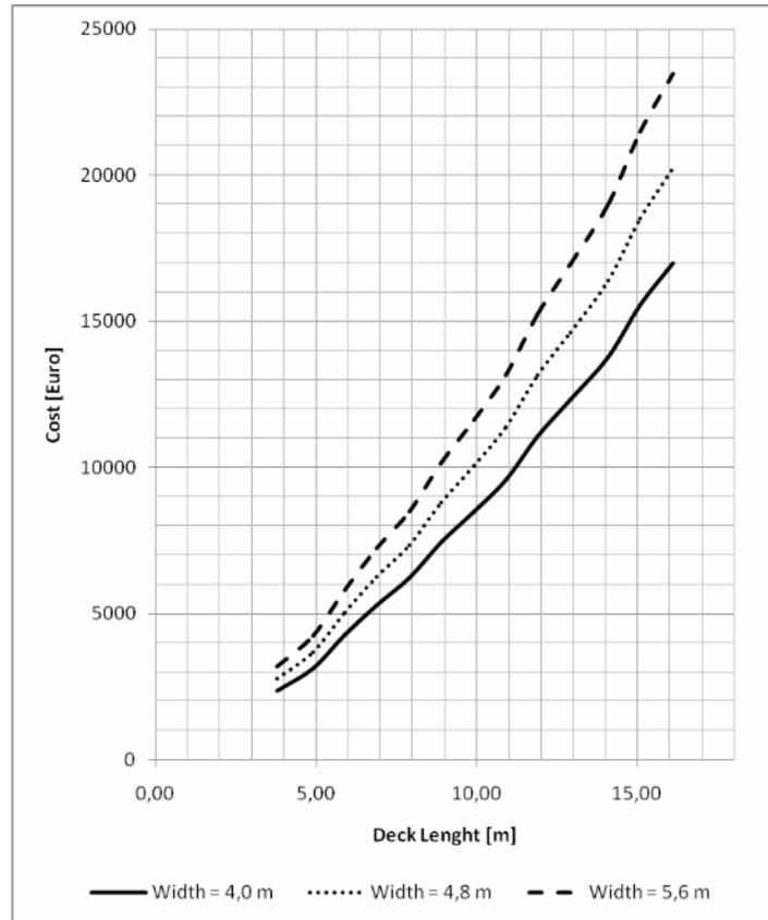
Fig. 5. The cost of glulam decks, in function of width and length
