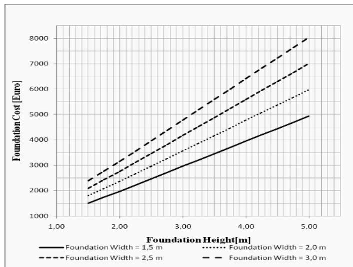
Fig. 8. Foundations costs in function of the dimensional elements
