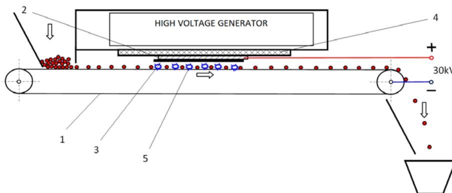
Fig. 4. The scheme of the equipment used for stabilizing medicinal plants, by ozonation
