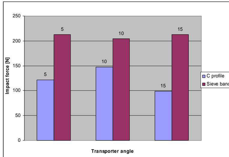
Fig. 5. *The impact force versus transporter angle*
