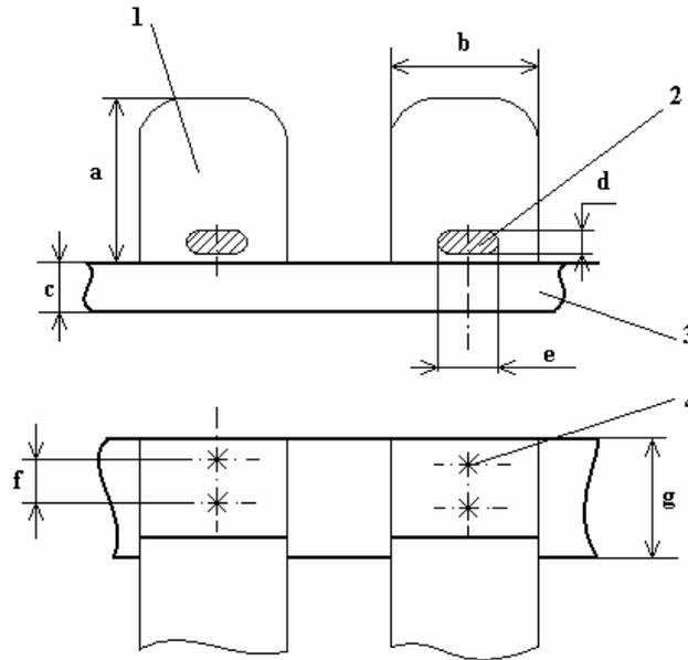
Fig. 4. *The Sieve band surface*
