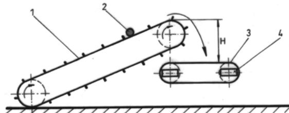
Fig. 2. *Modification of impact surface height*
