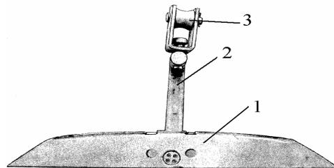
Fig. 1. A support for the main cable in case of the FP 2 skyline:
