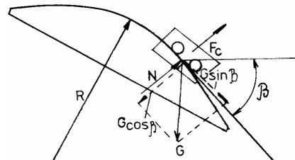
Fig. 2. *The scheme of the curvature radius calculation*
