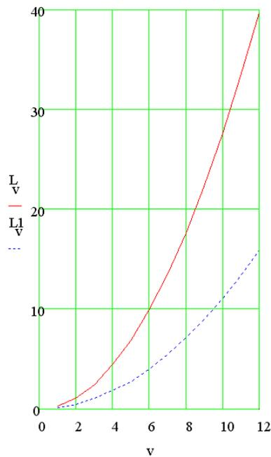
Fig. 6. The blade channel variation in function of the velocity for a braking angle of 16°
