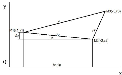
Fig. 2. Mathematical (computational) elements regarding the transversal section of a tractor road
