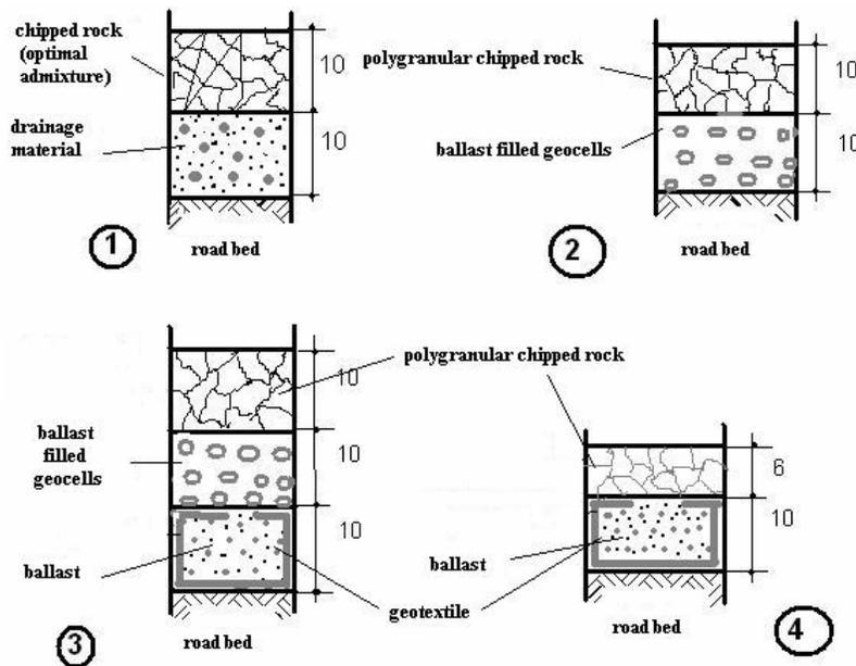
Fig. 2. *Experimental road sectors, with different consolidating structures*
