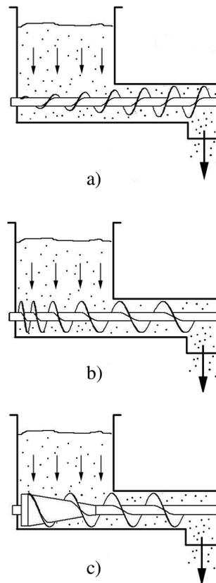
Fig. 1. Schematic representation of the uniform material extraction by variable geometry screw feeders: a) extraction using a tapered diameter screw feeder; b) extraction using a variable pitch screw feeder; c) extraction using a tapered shaft screw feeder
