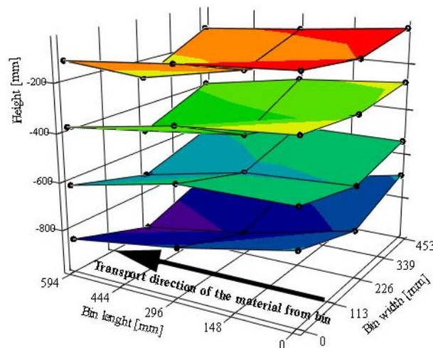
Fig. 4. *Flow profile of a wheat semolina discharged from a feeding bin with a screw feeder with variable pitch and constant screw flight diameter*
