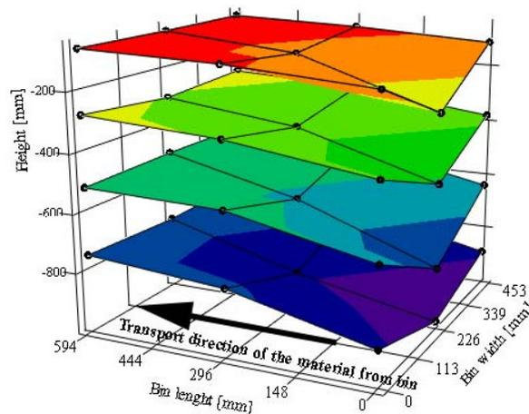
Fig. 3. Flow profile of a wheat semolina discharged from a feeding bin with a screw feeder with constant geometry
