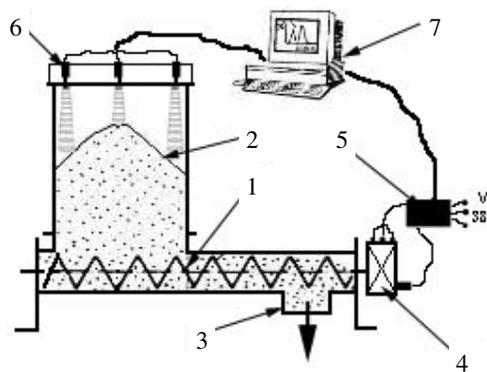
Fig. 2. *Experimental stand with horizontal screw feeders with variable geometry:*
