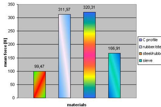
Fig. 4. Means of impact forces on several materials
